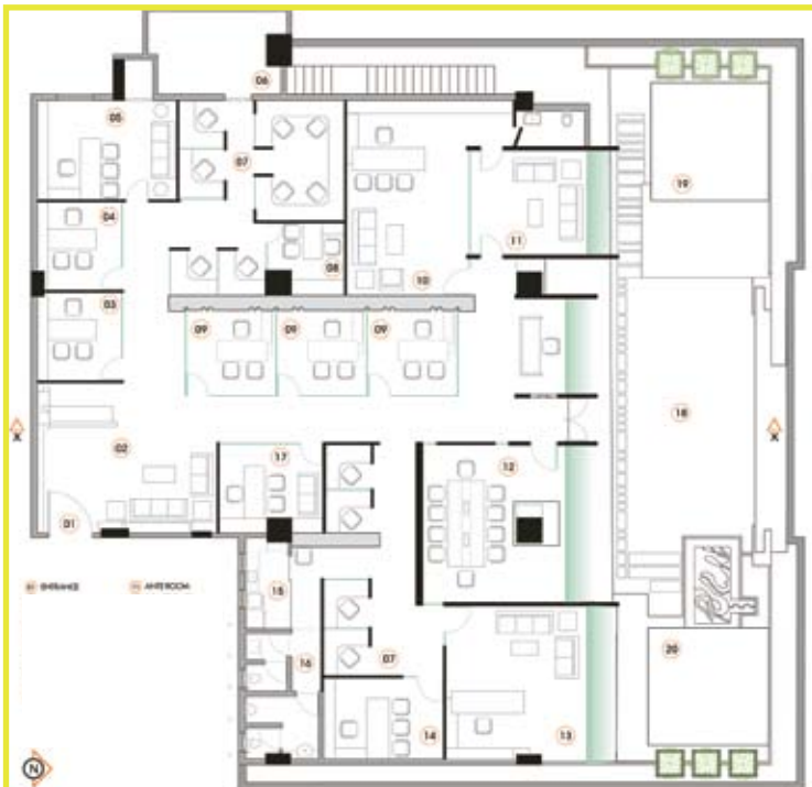
1 Entrance, 2 Reception & waiting, 3 Cabin 1, 4 Cabin 2, 5 Director's cabin 1, 6 Filing store, 7 Staff, 8 Cabin 3, 9 Sales cabins, 10 Director's cabin 2, 11 Ante room, 12 Conference, 13 Director's cabin 3, 14 Cabin 4, 15 Pantry, 16 Toilets, 17 Cabin 5, 18 Lawn, 19 Deck 1, 20 Deck 2.
